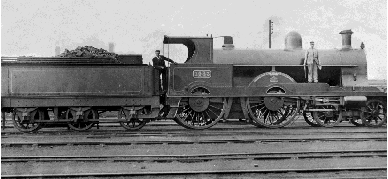
A 'Benbow' LNWR No.1943 Queen Alexandra with extended 'Precursor'-type cab and outside Joy valve gear; middle-height capuchon.
